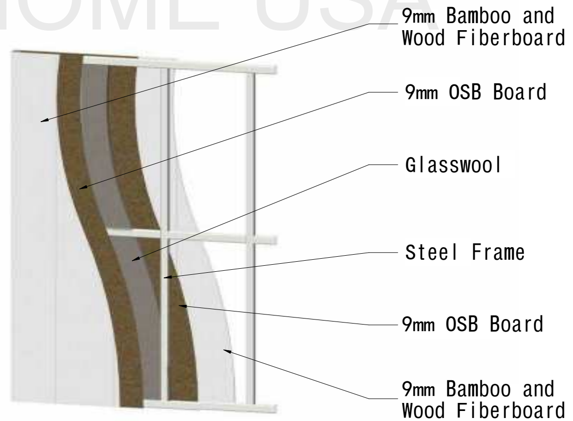
Section View of Interior Wallboard
